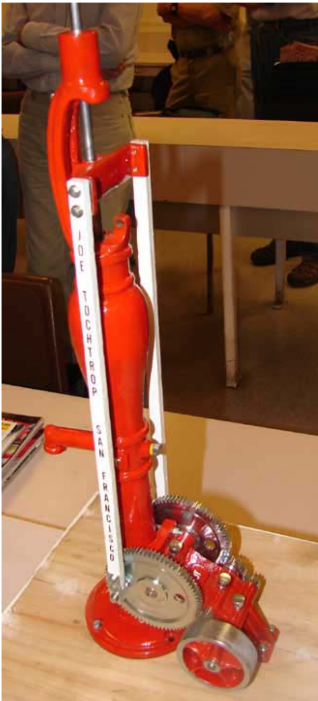
Joe Tochtrop has castings and drawings available for both a 12" and 18" pump jack kit. See him for details.
