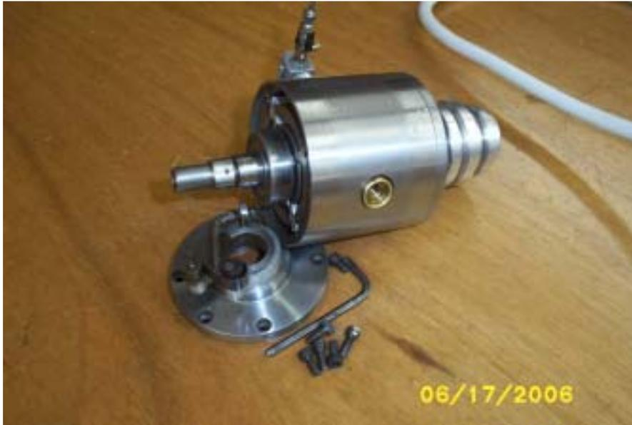
Al Vassallo's rotary piston engine. This is Al's own design; it is not a Wankel. The chamber was made by boring two holes on the lathe and finishing the shape between them with a shaper. The vane tip seals, not installed, are Teflon.
