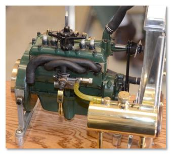
Dwight Giles showed us his progress on the Ford Model 'A' engine which now has a beautiful radiator, and a new brass flywheel based on the precise plans of a full-sized Model A. The completed wiring and electronics are tucked away in the base. To be completed is the exhaust manifold and muffler, as well as a Torrington bearing starter arrangement.
