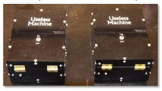
He also showed a pair of "Useless Machines". These black boxes sport a toggle switch. When pushed to the on position, a hatch opens and a finger emerges to promptly shut the switch off. If this engages your fancy, a kit is available at: frivolousengineering.com. Warning, the kit is not cheap at \$61.00 with shipping. As in government, useless ain't cheap.
