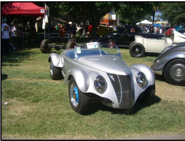
Jay's all-original midget roadster. Powered by a supercharged Ford V-8 60 mounted behind driver. Jay built the entire car including frame, suspension, even the wheels.
