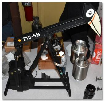
Tim Horn displayed an oil field "nodding donkey" pump to connect by a belt to his "Odds and End" hit and miss engine. The oil field terms "horse head" and "equalizer" cropped up, and were explained by Tim. He used an eccentric bushing that he was able to rotate to accurately center a shaft. For the making of custom O-rings, he used Loctite 404 to join the ends. A butt joint worked well, but some members recommended a scarfed joint.
