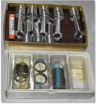
Dwight Giles showed us connecting rods and pistons for a Black Widow V-8 he wants to finish. The use of 2024 or 7075 aluminum is essential for the rods. No lubricant is needed for 2024 aluminum.
