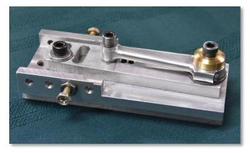
The fixtures for holding the rods were shown and explained. Round-over bits are used to contour the rods, which are "flipped-over" to machine the opposed side.
