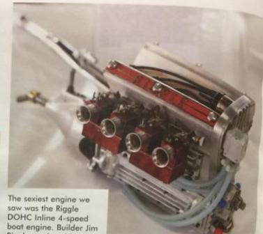
The sexiest engine we saw was the Riggle DOHC inline 4-speed boat engine. Builder Jim Riggle produced his own patterns and molds for the water-cooled DOHC monoblock engine.
