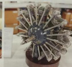
Arizona's Paul Knapp built this 1/4-scale Pratt & Whitney "Wasp Jr." 9-cylinder radial aircraft engine. Paul estimates that the engine's 15.8 cubic-inch displacement will produce over ten horsepower at 4,000rpm!
