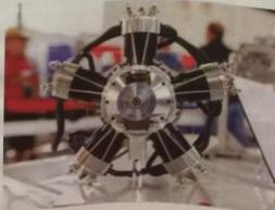
Here is the 1/2-scale Edwards 5-cylinder radial model aircraft engine. Designed and built by Forest Edwards, the 5-cylinder radial burns regular gasoline, incorporates a dry sump lubrication system, and produces more than six horsepower!
