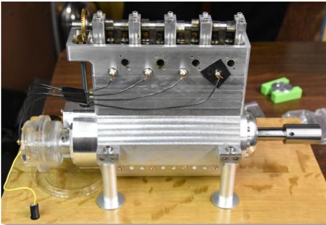
Peter Lawrence had first pops (about five seconds) from his “test mule” engine. It is actually a lovely, original, four-cylinder in-line gem. It uses a single overhead camshaft driven by a bevel-gear vertical shaft. He is currently sorting out ignition problems, with his Hall-effect system sensors flaming out regularly. Paul Denham mentioned that he uses reed relays to avoid that problem
