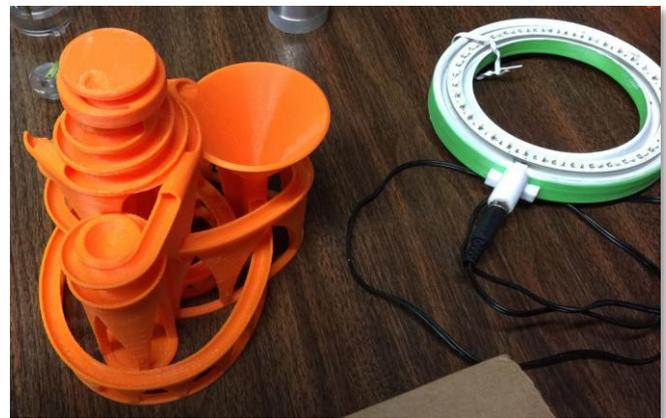
Continuing with his 3 D printing, Mike has continued to refine his magnetically held ring light (based on angel lights) for Bridgeport mill spindles. He has also made a fixture for an inexpensive light bar magnetically held. Next he built a gravity marble toy, a plan holder for the Bridgeport mill, and a variety of other projects.
