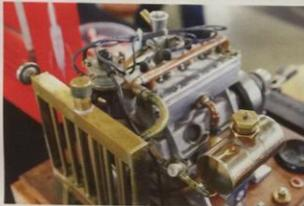
Lots of cool brass fittings, radiator and fuel tank adorned this 1/3-scale Wall 4-cylinder model engine.
