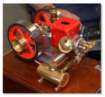
Dwight fired up his re-design of the old Upshur Farm Engine, the GEM 1. Three of these are being built and will be the subject of a build article in "Model Builder Magazine". It's a much improved design over the original. It is a throttled engine, not a hit and miss. Jim Piazza has been "making parts" not an engine. This is for the legendary Offenhauser 270. He was given a smaller scale Offenhauser block from Georgia Model Products to given him inspiration for additional pieces.
