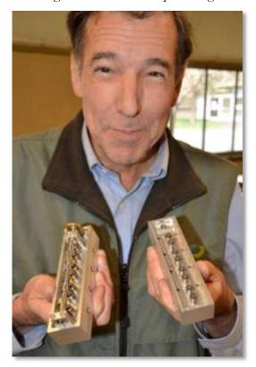
Peter showed us his latest version of a compression checker. This one works well, but sadly, it showed huge leaks on all valves tested. He then decided to press fit the valve cages, and that failed. He feels that it was due to distortion from the press. He is
