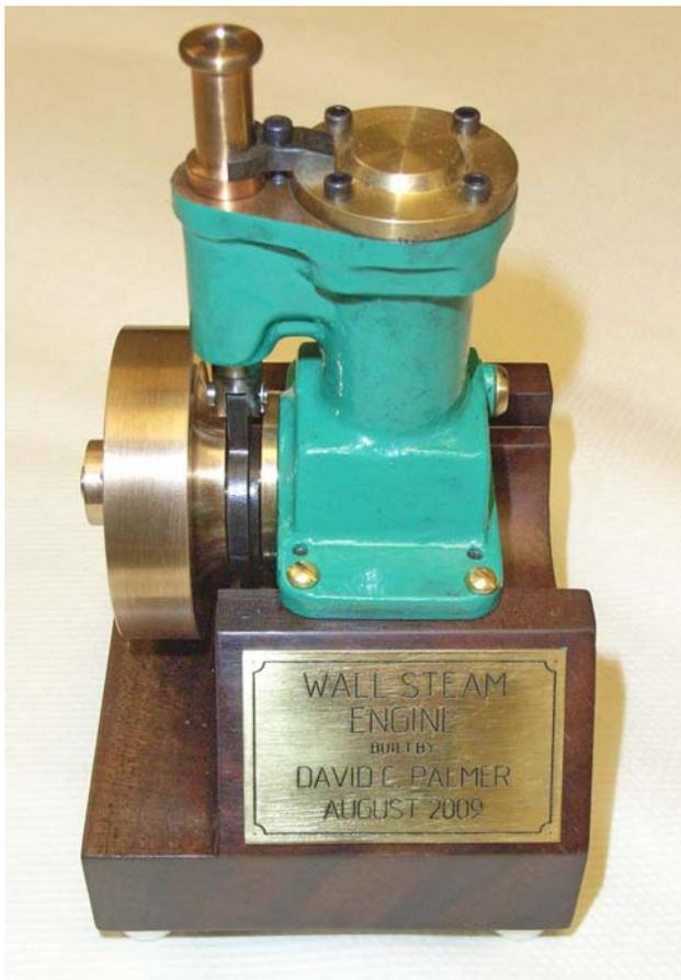
Well, the brass plaque says it all, well, most of it. It is not well known, but Elmer Wall did design at least one steam engine: the Black Knight. It features an 11/16" bore and 11/16" stroke and is still listed in Coles' Power Models.
