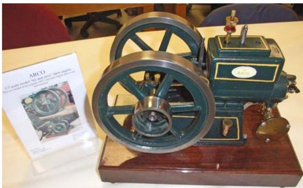
Shannon built this model of the 2 1/2hp Arco 1920 hit-n-miss engine from castings for the similar Economy engine by Joe Tochtrop. The two brands of engine were made in the same factory and shared many details.
