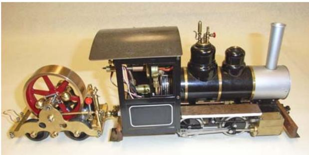
Dennis Mead's G scale locomotive "Ruby" now has a load car which adds some drag to simulate a string of cars and also acts as a governor on a
