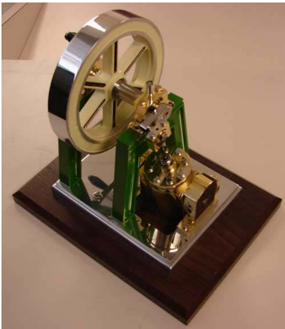
Rick Levesque's oscillating steam engine \frac{3}{4} " bore 1\frac{1}{2} " stroke Design by Rudy Kouhoup.
