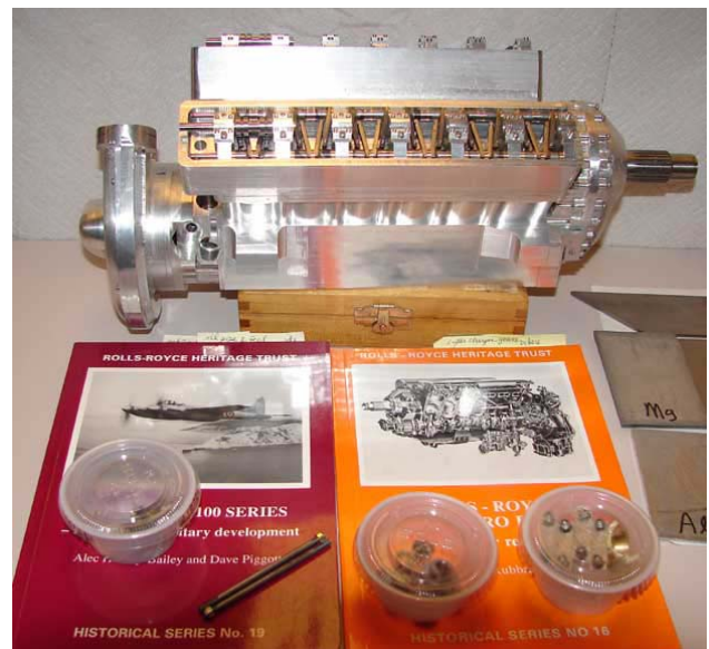
Peter Lawrence continues his build of the Rolls-Royce Merlin. This view shows the top of the
