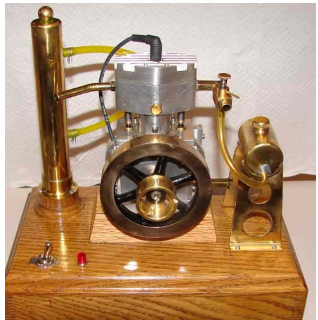
George Gravatt's model of the Palmer ZR-1 marine engine: design by Hamilton Upshur.
