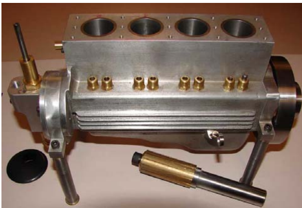
Dwight Giles 4 cylinder engine is one-half of the Black Widow V-8. Cylinder lap in front.
