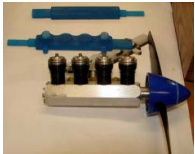
Jerry James: Four cylinder aero engine: fabrication in the front; patterns in stereo-lithography in the background
