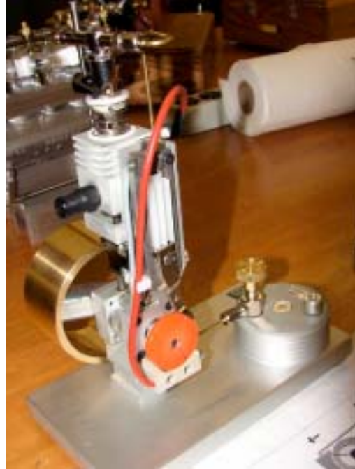
Carl Wilson's Dirod electrostatic generator: crank it up and make sparks
