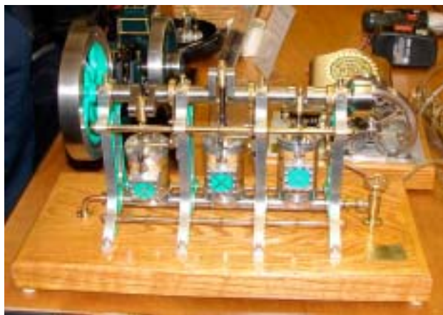
Dave Palmer's beautiful 3 cylinder version of a 1 cylinder Coventry engine published in Live Steam
