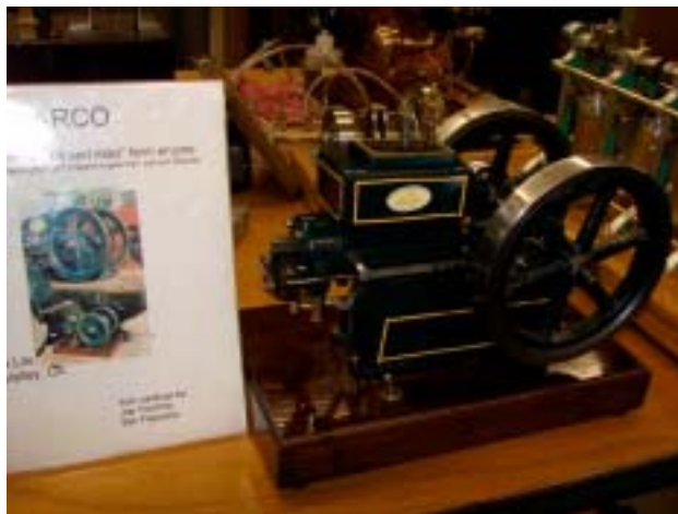
Dave Palmer's beautiful 3 cylinder version of a 1 cylinder Coventry engine published in Live Steam
