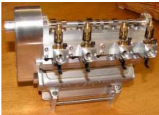
Dick Pretel's OHC conversion of the 50cc Wall 4
