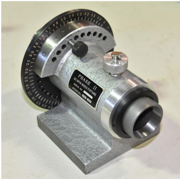
Carl Wilson showed a spin indexer he had reworked by reversing the spindle for better operability.
