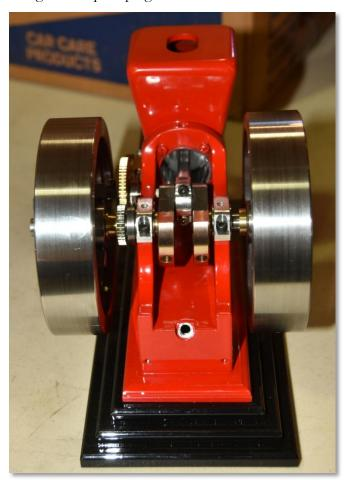
He followed a procedure detailed in Model Engine News (MEN) to balance the crankshaft. The formula for balancing involves weighing the
