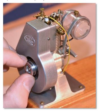
Next shown was a George Luhrs original single cylinder "Briggs and Stratton-like". This tiny gem is only .074 cu. inch in displacement. The bore is around one-half inch. The miniscule fuel line is fashioned by stripping the insulation from a single-strand copper wire. Paul mentioned that Teflon insulated wire will furnish a "tubing" supply that will hold up better to gasoline. Mr. Luhrs said that machining the tiny valve stems was a major challenge.
