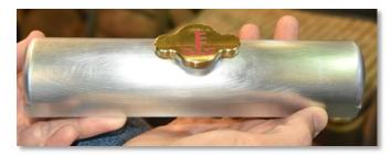
The 6061 aluminum tank top took eight hours on his three–axis Bridgeport CNC machine. The filler cap is threaded, right up to a shoulder.
