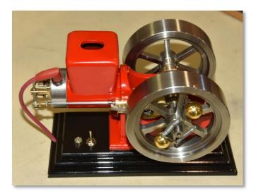
Paul Denham showed his latest touches on his modified GEM horizontal single. His original hit-and-miss mechanism, with the lockout arm, works well at low rpm's. He is using a piezo coil to energize the spark plug.
