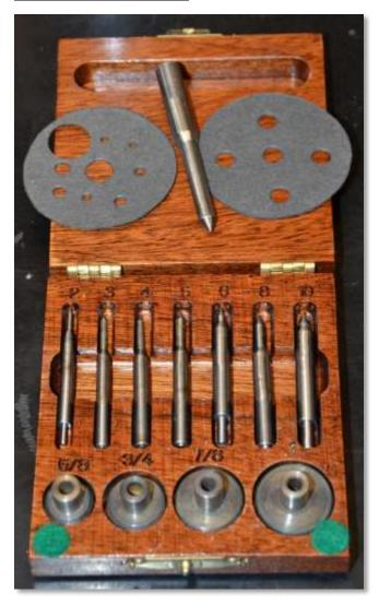
Dwight Giles made a new set of gasket cutters up to one-inch diameter. Mike Rehmus made a very nice custom wooden box to showcase this latest version. It will all be fully detailed in Model Engine Builder in issues to come.
