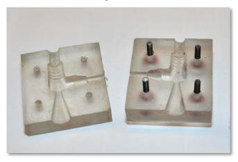
The resin is weighed 1 to 1 with a digital scale then mixed taking care to minimize air bubbles. The mixed resin is poured into the conical sprue: Dwight prefers a clear resin for the mold so that air bubbles may be seen. He loosens the screws slightly during the pour to vent the air in the mold then tightens them during the cure. The boots are de-molded after 5-7 hours but they are still soft so they are hung freely rather than being laid down.
