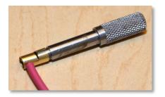
The wire is soldered into the brass terminal and the core pin (steel) is pushed into the terminal. The
