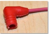
get all the details right. For the Black Widow V-8 engines by Dwight Giles and Ken Hurst that means custom molded spark plug wires. Dwight brought all the fixins for his Tech Topic and showed us how to make spark plug boots.
