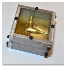
The boot pattern in the middle was made from two "L" shaped ¼" thick brass pieces soft soldered together. Dwight first tins the one face of each piece and then solders
