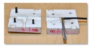
The finished pattern board is clamped into the flask (mold frame) and a rigid molding compound is poured in on one side. When this has cured the other side is molded. After curing, the mold frame is disassembled; the mold halves separated from the pattern board, and then drilled and tapped for screws.
