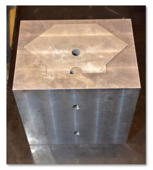
John Gilmore bought some lovely aluminum pieces from Roy Anderson and in the process met his son in his advanced machine shop. The result was the slicing of two Black Widow V-8 block profiles from large billets of aluminum with an EDM machine. Once the set up was made, it took about six hours to cut, and all with tolerances held within 3 or 4 tenths! A goodly amount of 0.010"brass wire was consumed in this operation.
