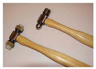
Dwight Giles builds a lot of different things and works wood as well as metal. The ball peen hammer head is 4130 steel – quenched, but not tempered. The mallet soft faces are nylon, and the handles are eucalyptus wood.
