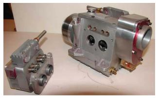
Jaime has his build of the Mastiff flat-four ready for assembly. Shown here are the crankcase and one of the cylinder blocks. Jaime drilled the crankshaft for lubrication and built a Hall Effect ignition trigger.
