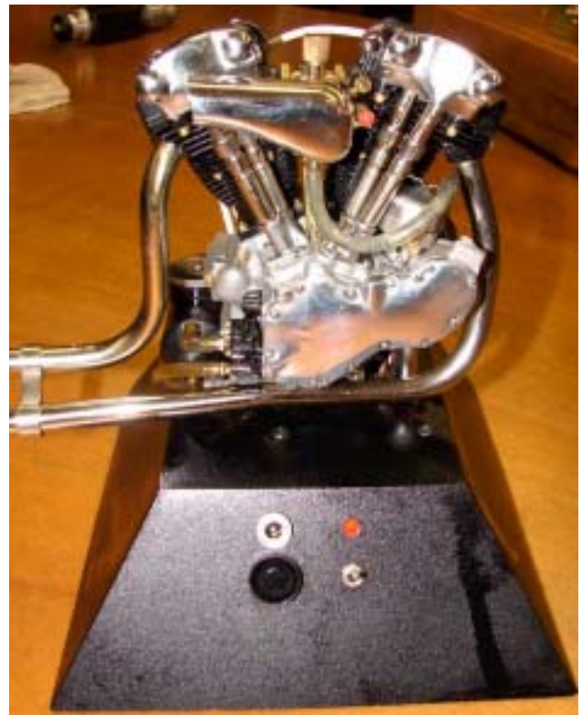
Bob Kradjian brought this model of the Harley-Davidson 1937 Knucklehead made by Replica Engines: http://www.replicaengines.com/ . One of the cylinders is loose because some of the cap screws holding it to the crankcase are stripped, but Bob started it right up.
