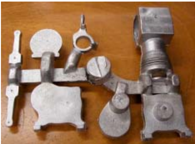
Don Catalano and John Vlavianos got together and designed this engine that can be built in several configurations. This set of castings, of course, would make a single cylinder engine, but Don pointed out that a second cylinder could be easily added. This casting tree is from the first pour: there are some changes to be made in the patterns and then it will be ready for production.
