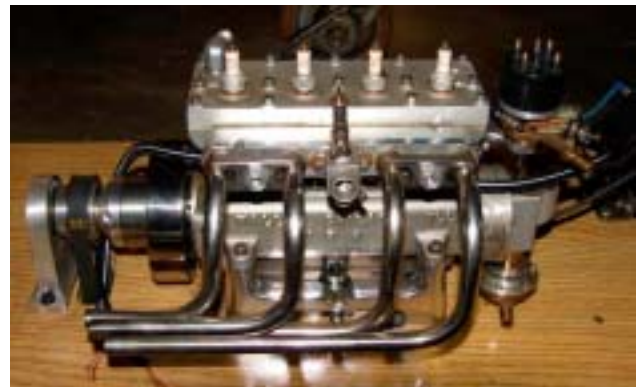
Paul Bennet built this Wall Four 50cc many years ago. Bob Kradjian now owns it, but it is going to return to Paul to be installed into a boat. Bob made a few changes: the small distributor cap and the electric starter driving onto the crankshaft via a sprag clutch are notable improvements.
