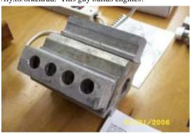
gest that you do also. You can read about its use in some of the automotive hybrid powerplants such as the Toyota Prius. George reports that he encountered trouble when he tried to mill the yoke without first making a clamping fixture. Seems the end mill got a little hungry for aluminum and crash.....!
