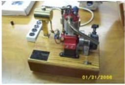
Ken Hurst made two of the Wall 30cc single cylinder 4 stroke engines. It features an 1 1/4" bore atop an 1 1/4" stroke and is fired with a 12 volt coil and battery system. The pull starter was an organ donor from a small chainsaw and is grafted on very nicely. Note the "gas tank on a post" which feeds fuel by gravity to the carburetor. Ken said that this arrangement guarantees that the fuel will leak out of the carb if he forgets to turn off the valve.
