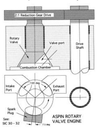
designed to produce more horsepower than any equivalent poppet valve engine. These large and very complex engines were completely superseded by turbojet engines in the late 1940's.
