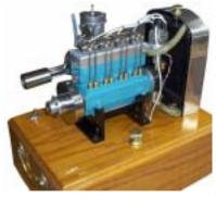
Dwight and Ken are making three Wall 4 engines converted to overhead valve. Some of the details:
