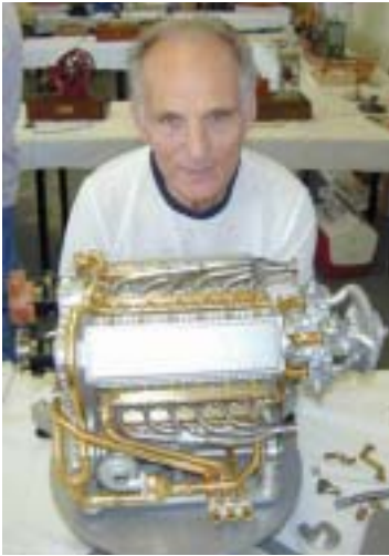
Clen Tomlinson is seen here at the 2003 Pacific Rim International Model Engineering show in Oregon with his nearly-completed Napier Deltic 18-cylinder engine.
