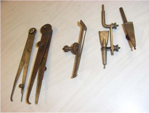
Ken Hurst displayed a variety of old measuring tools. On the left two hermaphrodite calipers (the British call them odd-leg calipers.) They are useful for scribing a line located from a flat surface. On the right are three lever type indicators: the movement of the indicator tip is magnified by a series of levers and displayed on a short scale.
