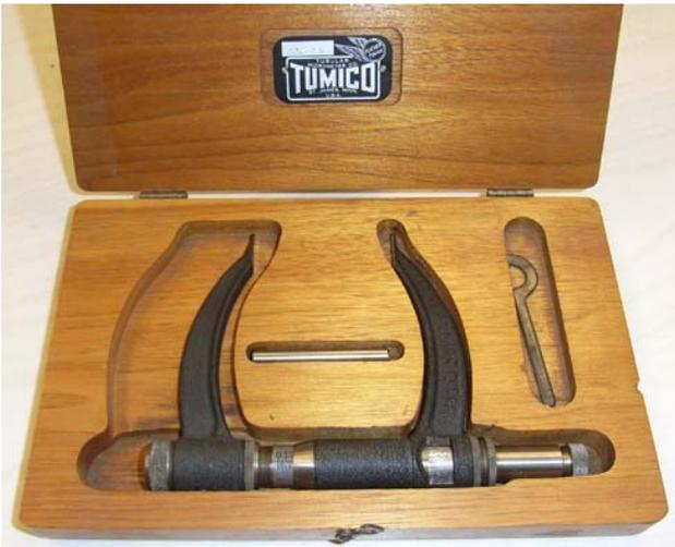
Bob Johnson brought his main bearing micrometer. The long reach of the anvils makes it possible to measure the diameter of crankshaft mains while the crank is in the block. I think the upper bearing shell has to be removed before measuring the journal.
