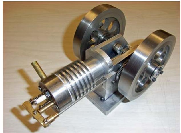
Mike Stimm built this Upshur Farm Engine from plans in Strictly IC. It runs on a vaporizing carburetor designed by Jan Ridders using Coleman fuel. Mike said it starts easily
