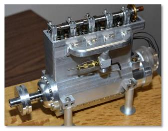
Peter Lawrence showed us his four-cylinder in-line engine that he is developing as a proof of performance. This is his first attempt at an internal combustion engine. He is making good progress on this build with excellent compression, working ignition system, intake and exhaust manifolds, a model airplane carburetor, and a functioning oil pump. The overhead camshaft is supported on five bearings. The brass bevel gear (4 to 1 ratio) to drive the cam looks possibly a bit small for the forces of
