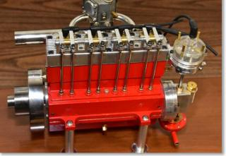
Dwight Giles brought us up to date on his modified Wall Four build. He completed the distributor incorporating a small lateral ramp to anchor the Hall effect sensor. The sensor can be attached with a short piece of shrink tubing for easy removal.
