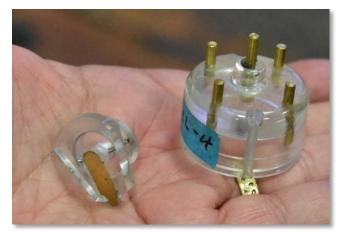
He passed around the nicely polished, clear acrylic distributor, cap, and rotor. Details of the stainless steel manifold TIG welding and bending process were presented.
