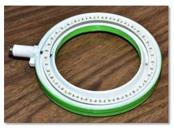
Finally, he is creating a LED ring light for a milling machine with his new 3-D Held to the machine by magnets. For the light source, he is using "Angel Eyes" cheaply available DX.com and with power supplies for only \$0.92!
