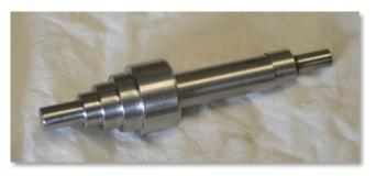
A clever stepped adapter was shown (see photo above). It allows the machinist to insert the device into a collet and move to other sizes without removing and replacing. This will be featured in an upcoming magazine article.
