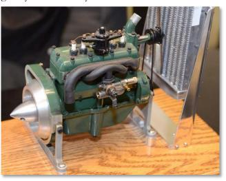
New member John Place brought his one-fifth scale Ford Model "A" engine. Dwight is fitting it with a running stand and an aluminum core radiator. The radiator is constructed with no solder or welds, just the amazing new E-120HP epoxies that work so well. Dwight made all new dies for the tanks. Also pictured is one of Dwight's fuel tanks with nearly invisible seams. The Model A is one of the fine engines made some years ago in the Ukraine. Investment castings used, are particularly fine.
