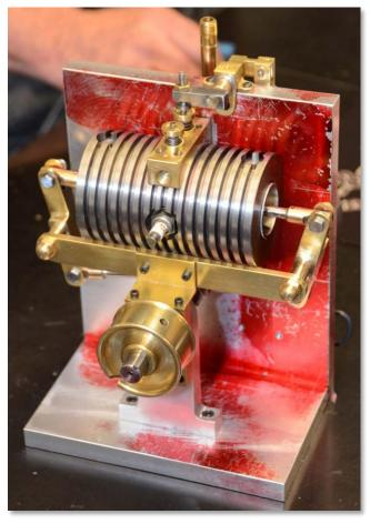
George Gravatt updated us on his original opposed piston engine. The valves are in place, the compression is 110 pounds, and it pulls good vacuum. The bore is an inch and a quarter, the stroke is two inches.
