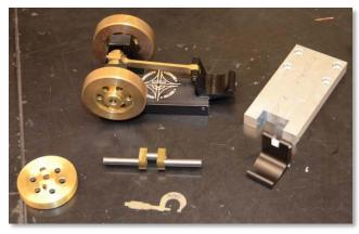
One of the nifty projects for the new facility is a "thumb treadle" to be made on CNC equipment. A pilot model looked and worked well. We use these devices at our shows to explain to kids how reciprocal motion is converted to rotary. An initial run of sixty thumb treadles is planned. Now if they just added a Torrington bearing? At the bottom of the photo is a tiny replica of a micrometer. It is labeled "HTEC" and was made in a stack of forty from 0.040" shim stock on the EDM machine.
