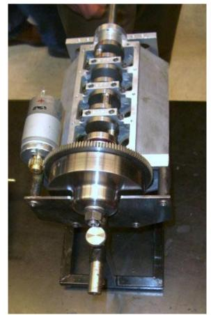
The starter motor is from an electric kiddy car. Dwight suggests buying the car then throwing it away after removing the drive motor. I wonder if one of Dwight's grandkids is wandering around the yard looking for his car. Oops, sorry, that's a bit off topic. Back to starter motors.
