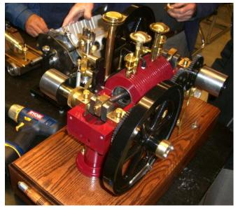
Lots of exhaust ports on this engine! On one side of the engine is a train of four large gears. I'm sure George will protect these from prying fingers before its run for the public. The entire project is nicely presented on a finger-jointed case with a shiny red automotive enamel spray paint job. You could think of it as a pair of Siamese-twinned singles joined the top of the head.
