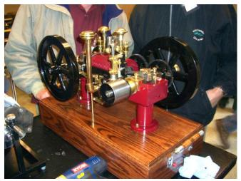
He incorporated an ancillary exhaust port at the end of the power stroke of each piston to port off excess heat. This, while robbing some power, results in an engine that will run for over an hour at only140 degrees. The two central paired exhaust stacks are capped by Dwight's innovative exhaust covers.
