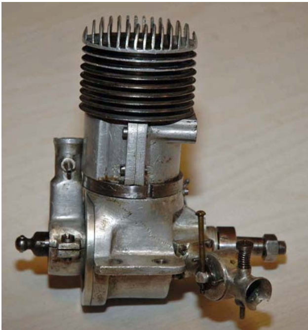
Bob Kradjian purchased this “what’s-it” engine at a collectors’ meet. It is an unusual design with no identification on it. Intended for a boat, it has two intakes; the intake with a throttle is visible at right-front. The engine is missing the piston and connecting rod.
