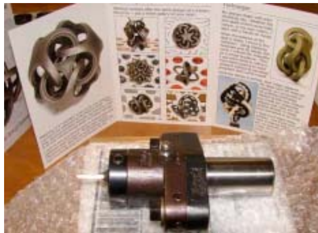
Steve Jasik says, "It's about time that I won one of these!" This is an offset rotary broach and Steve has been trying to win one of these for at least a year. What does it do, you ask? Well, it makes odd shaped holes. The tool is
