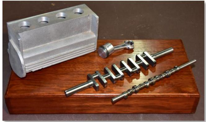
Paul Denham and Dwight have also been collaborating on "1/2 Black Widow" conceived as a 4 cylinder prototype for the V-8 version. Paul had the crank shaft and a cam shaft completed.
