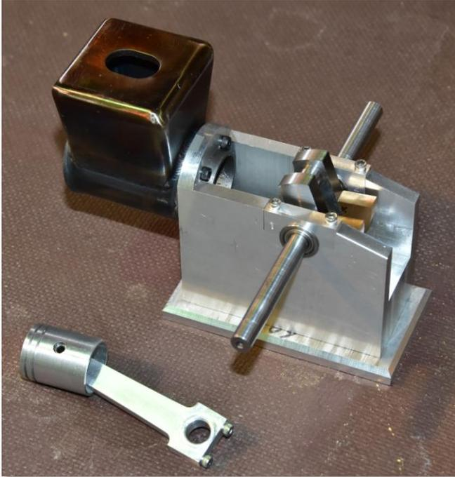
Larry Zurbrick showed progress on his GEM-1. He had the hopper mounted to the base with crank, rod, piston, and sleeve machined.
