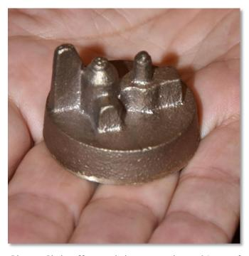
Glenn Christoffersen brings up the subject of holding small castings for delicate machining operations. The use of Wood's metal, epoxy spuds, or casting resin was discussed.
