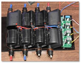
All of this uses the knowledge that our flat crankshaft fours and V8's all feature two pistons coming to top dead center simultaneously---one on compression, the other on exhaust. So, with a single magnet and four equally spaced sensors, you will be firing two spark plugs each 90 degrees. The exhaust spark will be "wasted" and of no significance. This amounts to just one magnet and four sensors, either Hall effect or reeds.
