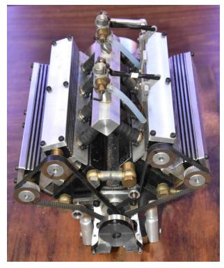
It was decided to drive a magnet wheel directly from the crankshaft. The sensors would be either Hall effect sensors, or reed switches. A single magnet was mounted in an aluminum disc. Paul then made up a Hall pickup ring with four sensors. He then created an ignition board with eight (yes, 8!) big, honking automotive coils. These came from China at
