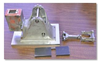
Paul Denham showed the Atkinson castings he received from Dwight Giles. The casting kit was made by Joe Tochtrop. Paul is proceeding very carefully since the castings are irreplaceable and delicate. He has modified the bearings from plain bearings to needle bearings.
