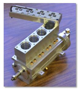
Dwight Giles updated on his Wall 4 engine progress. The head is made of 7075 aluminum. He hasn't put the ports into the head and may put them on one side. The fins are evenly cut which necessitated making the width of cylinder head 1/16th of an inch wider than the block in order to have fins align to the edge of the head. Dwight bored the water jacket in the block using his lathe by attaching the block onto a faceplate and using a boring bar.
