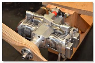
Jaime Quevedo has deftly re-engineered a German flat six air-cooled "boxer" into a four-cylinder version. Bore and stroke are both 25 mm. The internal tolerances are very close in this compact aircraft style engine. He used the designer's protocol for piston rings, but has not been happy with the results so far. The design uses a unique split crankshaft. The split in the crank is cradled and supported within the center bearing.
