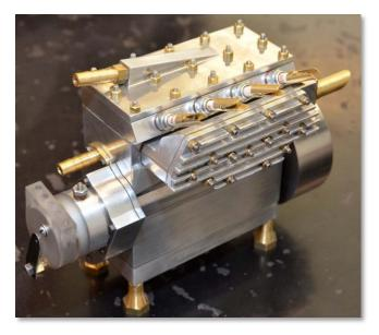
Joel Cohen continues his steady progress on the 15 cc Seal engine, this one machined from solid. It is developing into a lovely engine. His fit and finish is excellent. He is working on a carburetor now based on a gifted carb from Dick Pretel. When completed, this will be a largely original engine based on the English design.
