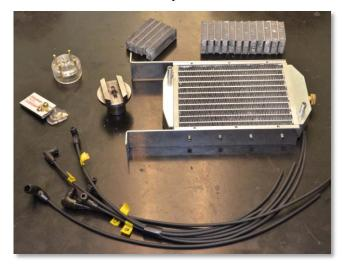
Dwight Giles has built another radiator "all glued together" with LockTite HP-120. These tiny marvels require no soldering or brazing. The temperature range is more than adequate and these adhesives represent a modern solution to an old problem. These epoxies require some learning and a special applicator.
