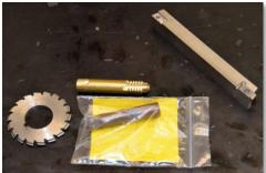
John Meridith is tackling two Eric Whittle designs at the same time. One is a flat four with a half-inch bore. The other is a single cylinder. Since they share a good deal of the parts, he is building them simultaneously. He needed 64 pitch and 32 pitch gears. He consulted with Jim Moyers at our last WEME show who recommended making a hobber and then cutting gears in his own shop. Jim also
