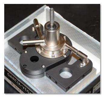
Jim Freel brought us up to date on his Black Widow V-8 project. Continuing on the theme of making the small bits first, he has finished the water pump. It is up to his usual high standard, and is nickel-plated. The nickel gives a nice, soft luster when compared to chrome plating. He used a lip seal found on the McMaster-Carr on-line catalog to prevent water drips.
