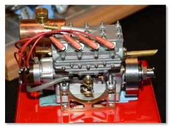
Joel Cohen did get his Seal to run, but not well. Despite this, he said: "I don't know when I've been so happy!" To alloy his happiness, he also noted a water leak into the oil. He is considering rebuilding the engine with a new block machined out of solid.
