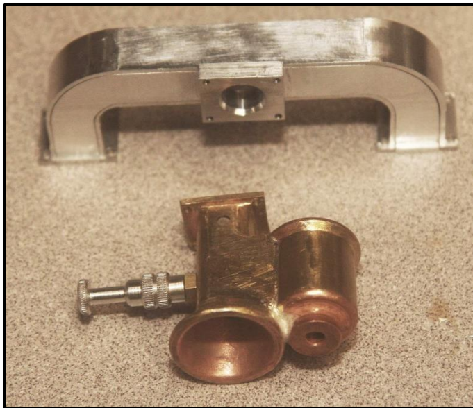
Intake manifold and brass carburetor.
