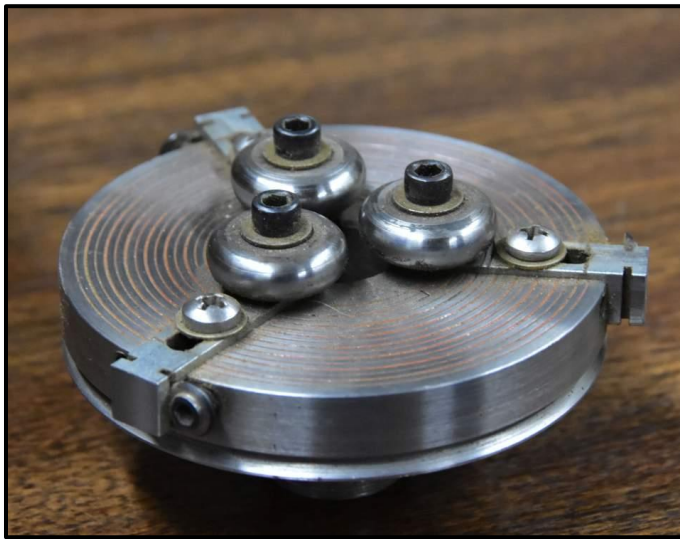
Fixture for swaging taper in brass tubing.
