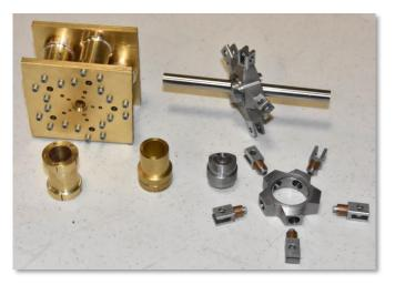
Peter Lawrence showed us a linear five-cylinder steam engine he is working on. It utilizes a swash plate connected to a drive shaft. It also has spider gears and a hub as well as multiple axial connecting rods. It will use a rotary valve to shuttle pressure between the two steam chests.
