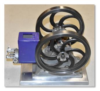
Paul Denham showed us his version of Joel Tochtrop's Atkinson cycle engine. He changed the taper mount to a collet arrangement for mounting the flywheels. Since there were no counter weights on the crankshaft, Paul developed his own brass counterweights that appear to nearly perfectly balance the complex Atkinson actions.
