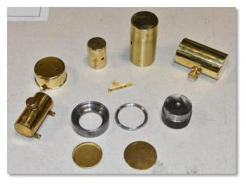
Dwight Giles gave us a masterful explanation of how to make his beautiful gas tanks. The ends are formed with dies that are pressed and the edges trimmed on a lathe.
