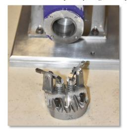
Pat O'Connor used Alibre to replicate a supercharger wheel for a Pratt and Whitney engine. He then sent it to Mike for 3D printing. He finished it using a slitting saw and a rotary table to cut the blades.
