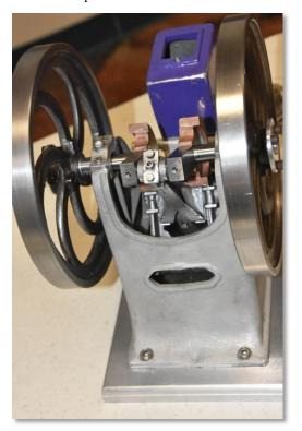
Paul used titanium for the pushrods and rocker arms to reduce reciprocating weight. He is willing to admit that small titanium shavings blaze up brightly. Don't ask how he found out. The body castings are thin and easily warped. He is using a nice flat metal base to keep everything lined up.
