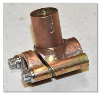
He also showed us a worn cross feed nut for his Clausing lathe that he rebuilt to be an adjustable nut that will not require replacement.
