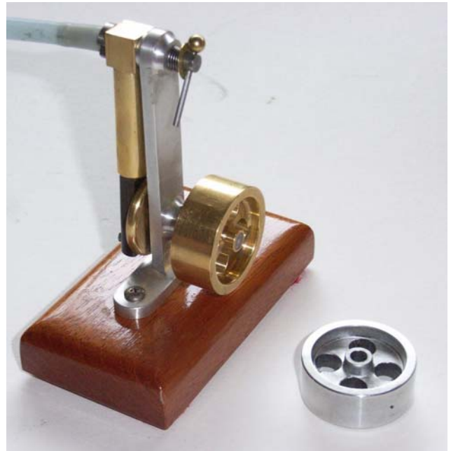
This is Dwight Gile's build of Radlett. The brass flywheel was turned from bar stock; the Zamak flywheel is the only successful casting from his aluminum permanent mold that was shown in last month's newsletter.
