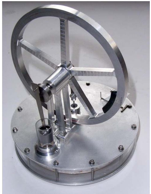
Peter Lawrence's low delta t Stirling engine will run- if he puts boiling water under the displacer and ice on the top. There are a few problems to fix: thermal short-circuit between the top and bottom plates and air leaks between the plates and the acrylic cylinder are possible reasons for the poor running.
