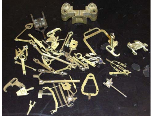
Jaime has received one of three sets of castings for the Cirrus aero engine which were made in Italy.
