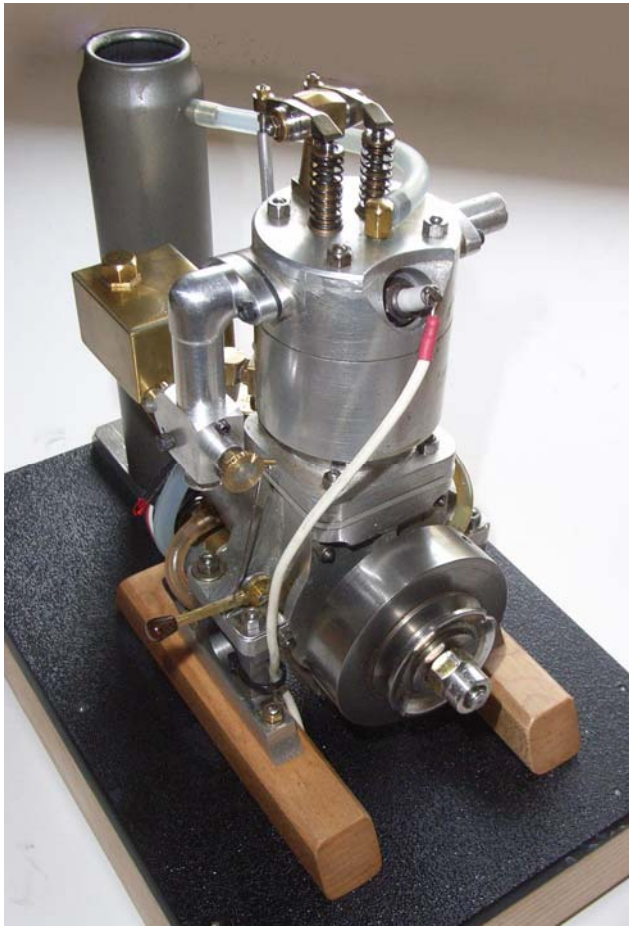
This Wall 15cc single is Bob Hettinger's first engine, made 40 years ago with castings from Cole's Power Models. It features ball bearings, internal scavenger type oil pump, and an external water pump.
