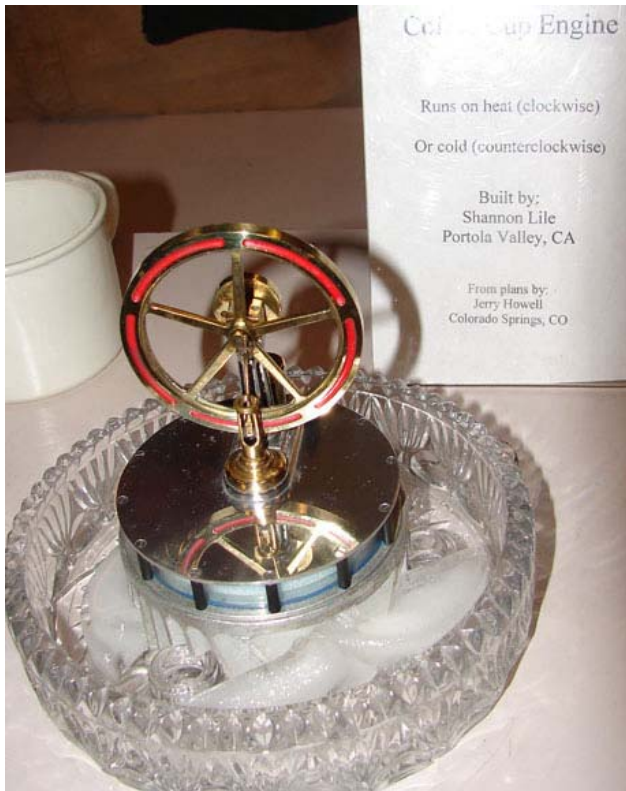
Low delta- t engine by Shannon Lile; Coffee Cup Engine
