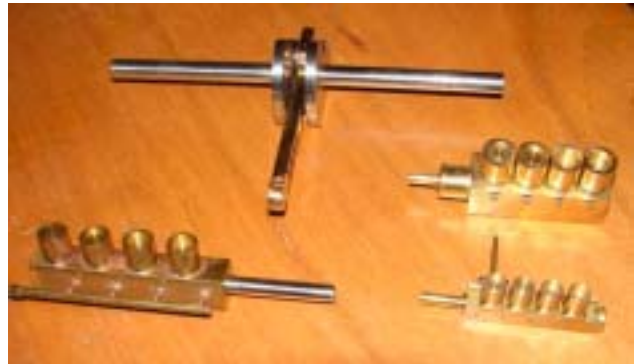
At the top of this photo is the crank and connecting rod for George Gravatt and Dwight Giles' latest project, the Red Devil. George drilled the rod 3/32" diameter from the crankpin bore to the wrist pin for lubrication. Cylinder blocks by Jerry James ?
