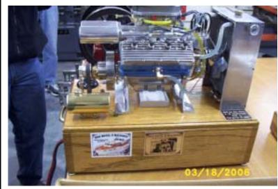
Ken Hurst built this Challenger with castings from Coles' Power Models in 1999/2000. Sitting on top of the manifold is two Walbro carburetors ( two one's in the hot rod parlance.) These carbs were designed for use with small two stroke engines that used intake vacuum pulsations to operate the fuel pump. The constant intake vacuum of the 8 cylinder 4 stroke engine will not operate the pump so Ken installed a low volume/low pressure Purolator fuel pump to mimic the operation of a single cylin-
