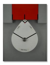
And the line of contact between a circle and a flat surface is at right angles to the flat surface.
