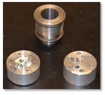
vertical height. He used 1144 stress proof steel for the cylinders. He used an Iscar parting tool for machining the deep fin slots with a nice rounded end to reduce stress. He is putting his Merlin V-12 project "on the shelf" for a time before fully launching into the camshaft phase of the build.
