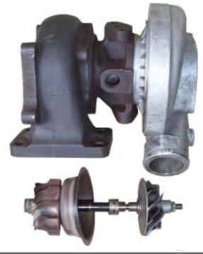
A supercharger that is driven by the exhaust gas is called a turbocharger, turbo for short. In the picture on the left, the major castings are at the top and the rotor has been removed and placed below. The hot, pressurized exhaust gases enter the exhaust turbine (left side of picture), and spin the rotor at speeds of 20,000 to 120,000 rpm. The intake air is compressed by the impeller on the right and flows into the intake manifold.
