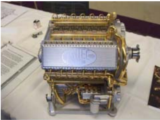
Napier "Deltic" 18-cylinder, 1/18-scale, opposed piston, marine engine developed by Clennell Tomlinson of Broadbridge, Heath, England
