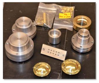
Dwight also showed us beautiful brass exhaust caps in three sizes. He presses the dome on the brass sheet with a custom made die and couples them to the base with six brass rivets on the smaller ones and eight on the largest. The ½ by 20 threaded coupler is silver soldered to the base. All is done with meticulous attention to detail. These caps qualify as mechanical jewelry.
