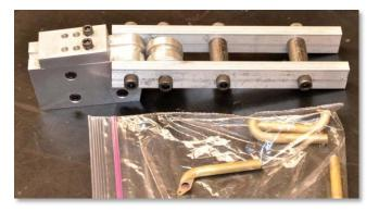
Jim Piazza has ventured into the world of tube bending. This time it was to make a water inlet pipe for his Offenhauser model project. He first
