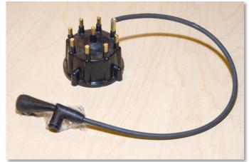
There is the first spark plug wire, without its distributor end boot. The cone shape at the left side of the boot is the sprue – the channel through which the rubber enters the mold. This excess material will be cut off. The cast distributor caps were from a vendor (Barker) in Florida.
