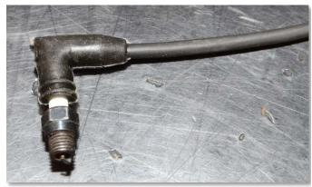
There is a minimum of flash to remove and Dwight says that it simply pulls off leaving a nice right angle spark plug boot.
