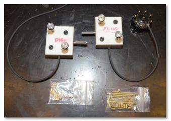
Dwight Giles continued the saga of his molded spark plug wires for the Black Widow V8 engine. Last month he showed 2 finished molds. During the intervening month he cast polyurethane rubber into the molds and brought them to the meeting for Bits and Pieces. He removed the two clamp screws, opened the mold and showed us the result:
