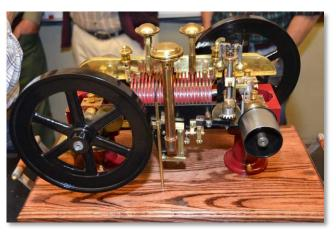
George Gravatt fired up totally original his opposed-piston design. He substituted fiber gears for the metal gears in the middle of the gear train. This resulted in а considerable reduction in noise. He also switched from the original hit and arrangement miss to throttle control. This engine attracted positive attention at the Palo Alto Show.
