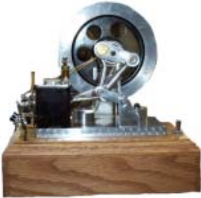
George Gravatt's Atkinson Cycle Engine
