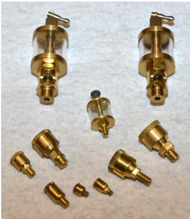
Dwight Giles made these grease cups and drip sight lubricators for his Upshur farm engine.
