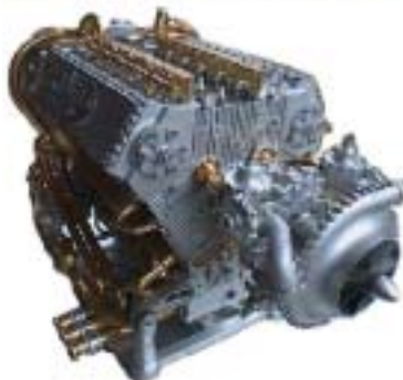
Clennell Tomlinson's 18-cylinder, 1/8th-scale, opposed piston, marine engine.
