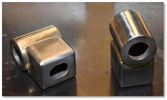
Dwight generously donated two cylinder and hopper assemblies that were silver-soldered together along with plans to complete the engine to club members who will pledge to actually build the engine. He recommends a five-thousandths taper in the sleeve, so that the sleeve contacts only during the last quarter inch of the press fit.
