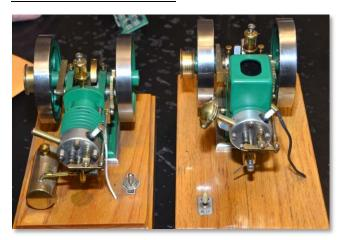
Dwight Giles showed two Upshur farm engines he fashioned about 12 years ago. One finned, the other cooled with a hopper. He discourages building the air-cooled version as the design resulted in flexing at the base of the cylinder. The hopper version is a far sturdier design and resulted in a fine-running engine. If the bore is increased to 7/8ths from 3/4 inch, the engine runs even better.
