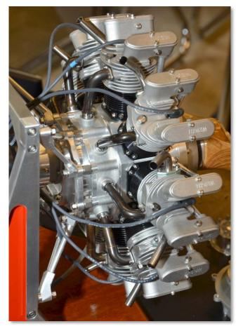
carburetor design that works well replacing a Super Tigre version. He says the engine starts easily with hand propping and runs well. John says the engine is too stiff for even geared-down electric starters. He started this project in 1992. Unfortunately the casting sets went off market about five years ago. The castings are of superlative quality and are chiefly of the lost wax type. Note the crisp lettering of "WRIGHT" on the rocker arm covers. The entire
