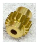
lower right corner of the first photo. The starter pinion is mounted on the shaft of a motor taken from a Tyco kid's car. Is one of Dwight's grandsons is wondering why his car no longer runs? The motor shaft has serrations, so the gear has to have them also.
