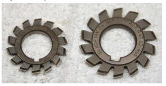
Two gear cutters are shown in this photo. These are involute gear cutters and come in sets of 8. Each cutter in the set will cut gears with a range of number of teeth so the number of the cutter must be matched to the size of the gear. This is, of course, in addition to the diametral pitch and pressure angle.
