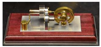
The displacer piston is aluminum and the power piston is graphite. Lyle Shannon wrote the nice description of the Stirling principles for the magazine article.
